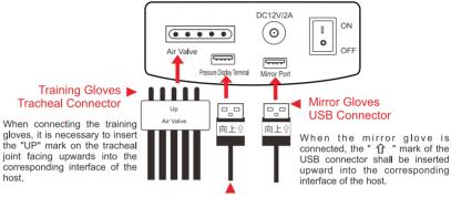
Pressure Handle When the pressure handle is connected, the " ① " USB Connector mark of the USB connector shall be inserted upward into the corresponding interface of the host
