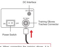
Note: When connecting the training gloves, it is necessary to rotate and tighten the tracheal joint clockwise to the corresponding interface of the host.
